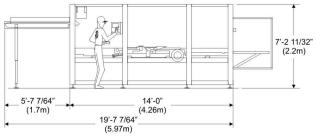
INSTALLED LENGTH BETWEEN CUSTOMER SUPPLIED CONVEYORS
