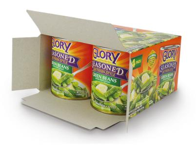
Produced on 24pt coated recycle board (CRB), this carton can self-palletize, withstand the rigors of shipping and distribution, and protect the product inside. The use of solid paperboard provides a superior alternative to the traditional choice of corrugate in club stores.
