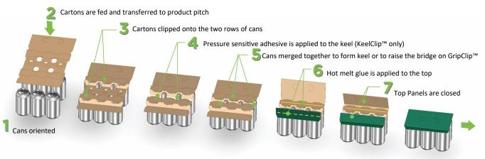
Can orientation system offers a choice of product orientation patterns that maximizes branding and obscures UPC codes. (Keel and ECO only)
