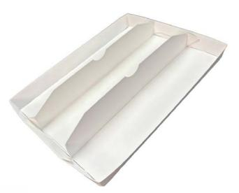
The TrayArray™ Lite paperboard tray has been designed as an alternative to plastic inserts to hold any type of cookie or cracker inside a flow-wrapped outer package. TrayArray Lite has foldable partitions which can be manually erected, or activated through automation during the de-nesting process.
